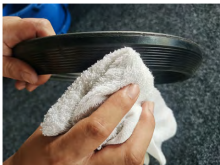
Cleaning the seal.
