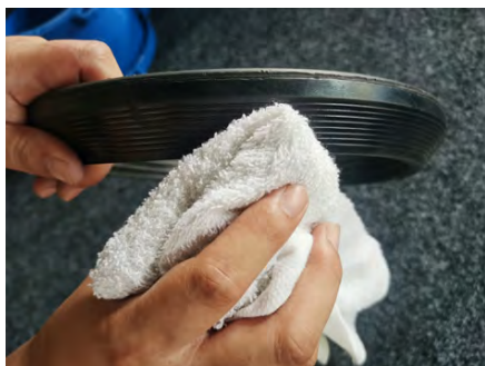
Cleaning the seal.
