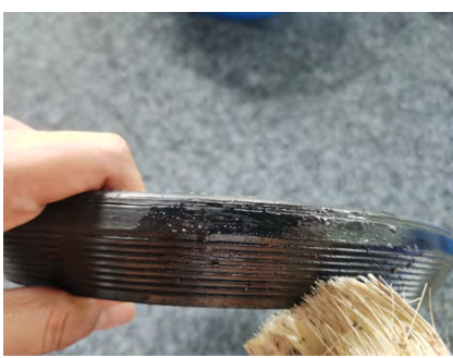
Applying suitable lubricant.
